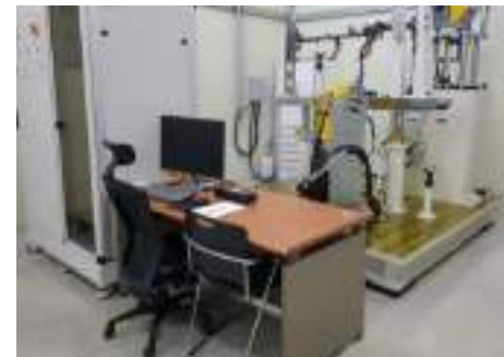
Cowl Cross Bar Rotational Durability Testing Equipment
